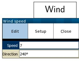
Wind vector estimated by XCSoar. Manual adjustment is possible with the connected InfoBox dialogue. Pressing the up/down cursor keys to cycle through settings, adjust the values with left/right cursor keys.
