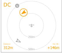
The three screenshots are taken in a sequence and demonstrate a typical near pass of e.g. two FLARM equipped gliders. The extra information is colour-coded in the already mentioned way. In the
