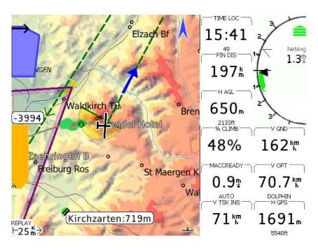
Figure 3.1: Typical XCSoar main screen layout
